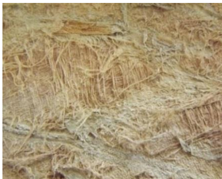
Figure 15. Side flesh of a tanned fish where the fibers are observed in a plane parallel to the surface and crossed almost 90^\circ layers.
