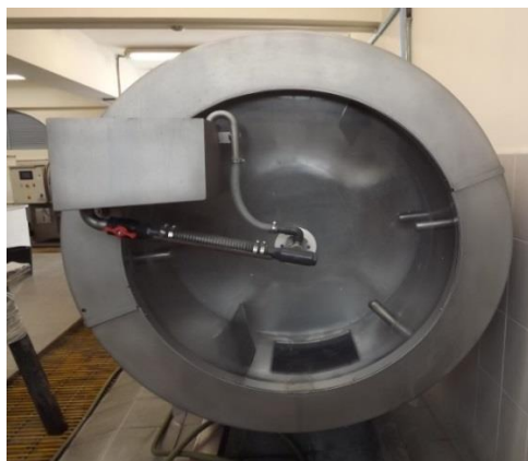
Figure 20. Tanning drum, made with stainless steel and clear acrylic face.
