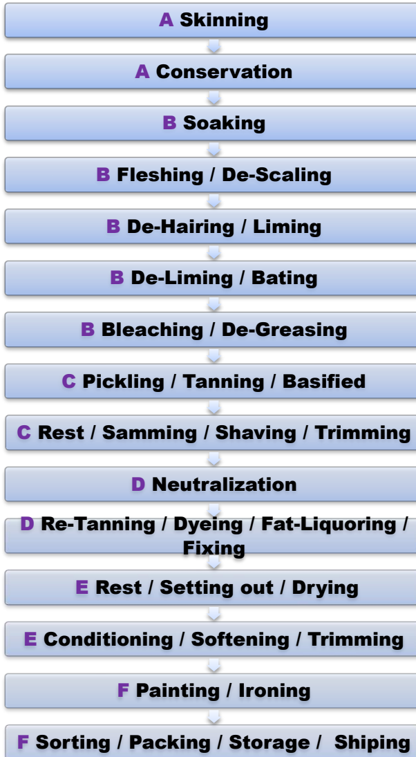
Figure 18. Diagram of tanning process.
