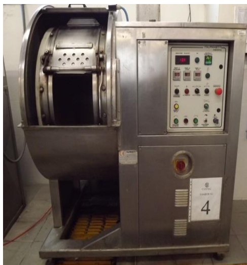
Figure 22. Laboratory (Reactor) stainless steel tanning drum with opened door.
