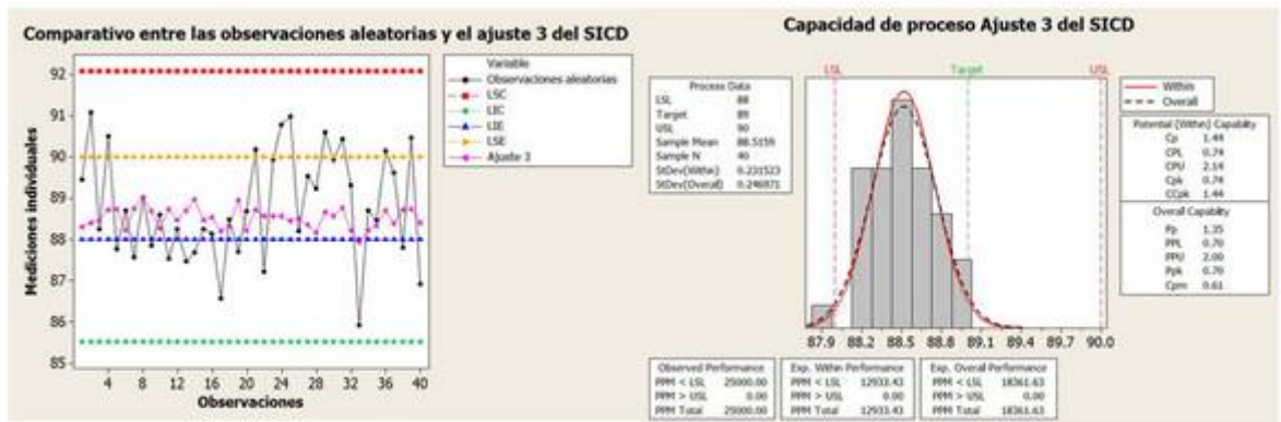
Image 11. IDCS Chart Control with specification limits required by the company and the process capacity for three adjustments, with a 1.44 Cpk.
