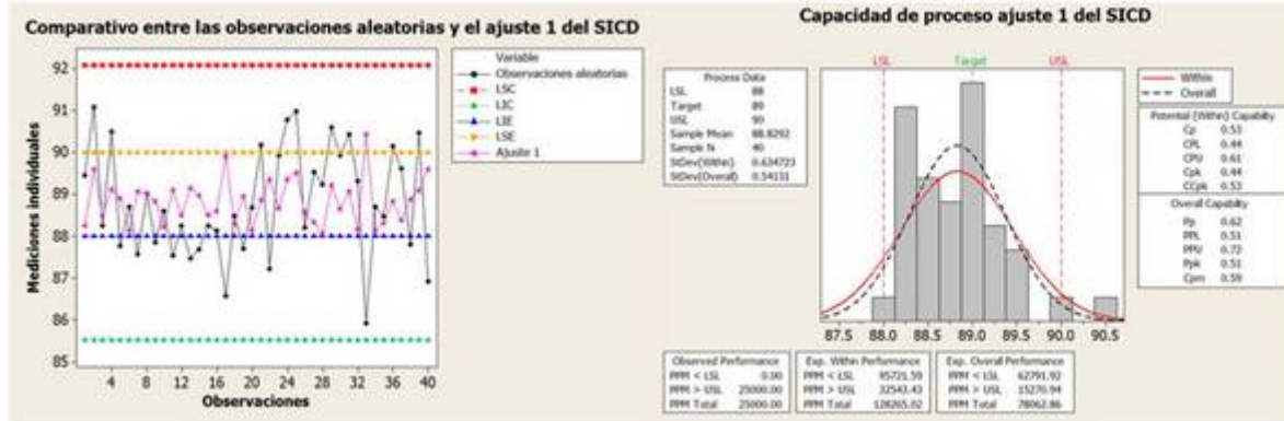
Image 9. IDCS Chart Control with specification limits required by the company and the process capacity for an adjustment, with a 0.53 Cpk.
