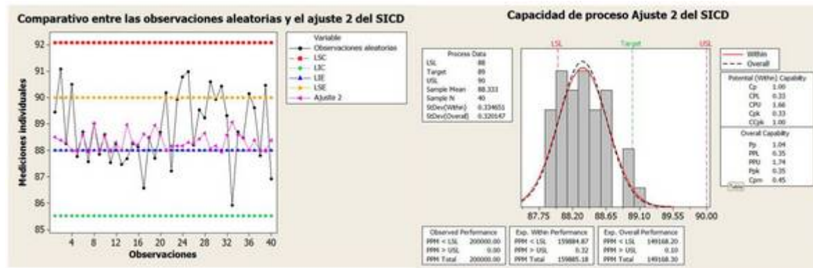
Image 10. IDCS Chart Control with specification limits required by the company and the process capacity for two adjustments, with a 1.0 Cpk.
